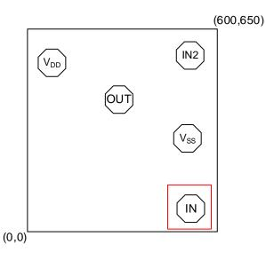
Note: The pad coordinates are given for the center of the pad, values in  $\mu$ m from the origin (0,0). Chip die size is 600 um x 650 um.
